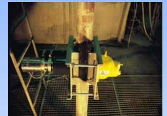
LB 444 Radiometric Density gauge with 90 degree clamp and mounting configuration.
