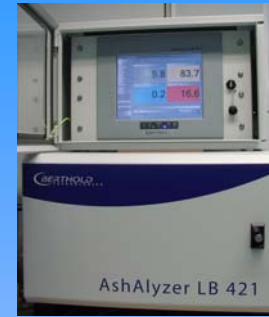
LB 421 showing color touch screen and CPU/electronics
